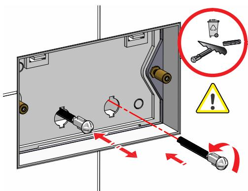
In order to let the water flow open and stop in the proper way, please adjust the actuators by screwing them in and out until the correct position is reached.
